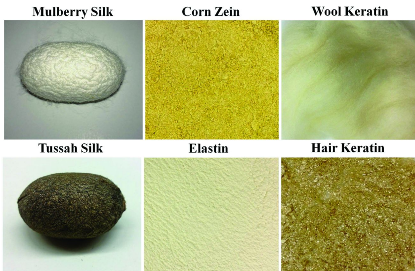
Figure 1. Natural proteins for composite materials, including various silkworm and spider silks (beta-pleated sheet structure), elastins (beta-spiral structure), wool and hair keratins (alpha-helical conformation and cross-linked by cysteines), zeins (alpha-helix structure), as well as collagens (triple-helix structure), resilins (beta-turn structure), and bee silks (coiled-coil structures) etc. (1).
